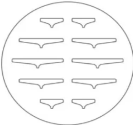
Equal percentage flow characteristic orifice
