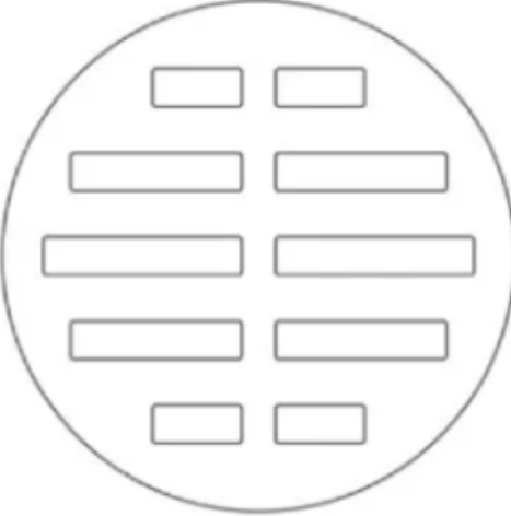
Quick opening flow characteristic orifice
