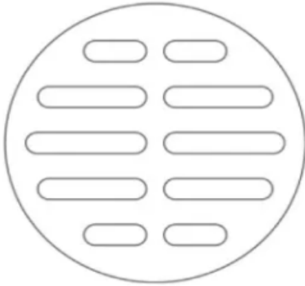
Linear flow characteristic orifice
